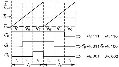
Fig. 4. 3-segment switching sequences of sector I.
