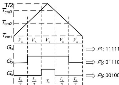
Fig. 3. 5-segment switching sequences of sector I.
