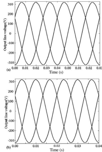
Fig. 7. Output line voltage in over-modulation region: (a)  $M=1.06$  and (b)  $M=1.16$ .
