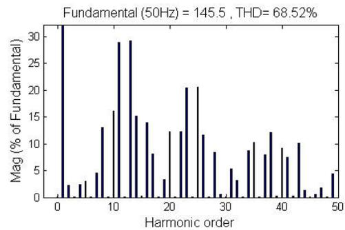
Fig. 9. Harmonics spectrum of 5-segment SVM with  $M=0.8$  and  $N=12$ .
