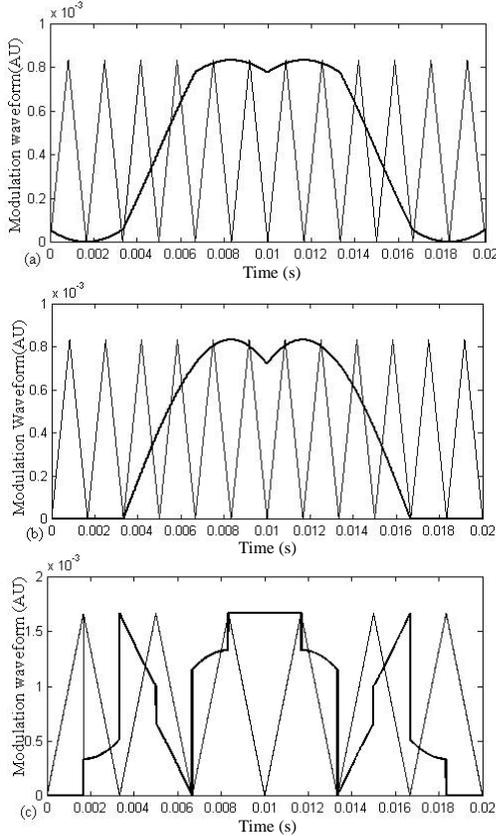
Fig. 5. Modulation waveforms of three SVPWM schemes: (a) the 7-segment scheme, (b) the 5-segment scheme, and (c) the 3-segment scheme.
