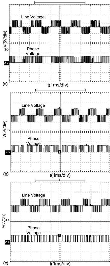
Fig.11. Experimental waveforms of DSP: (a) the 7-segment SVM, (b) the 5-segment SVM, and (c) the 3-segment SVM.
