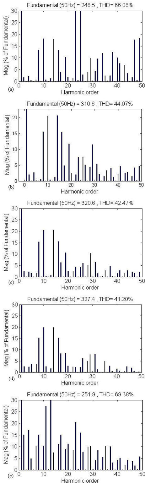
Fig. 8. Harmonics spectrum of 3-segment SVM: (a)  $M=0.8$  and  $N=24$ , (b)  $M=1.0$  and  $N=24$ , (c)  $M=1.06$  and  $N=24$ , (d)  $M=1.16$  and  $N=24$ , and (e)  $M=0.8$  and  $N=12$ .
