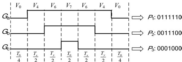
Fig. 2. Conventional 7-segment switching sequences of sector I.
