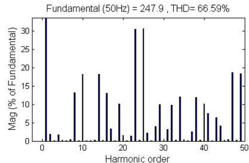
Fig. 10. Harmonics spectrum of 7-segment SVM with  $M=0.8$  and  $N=12$ .
