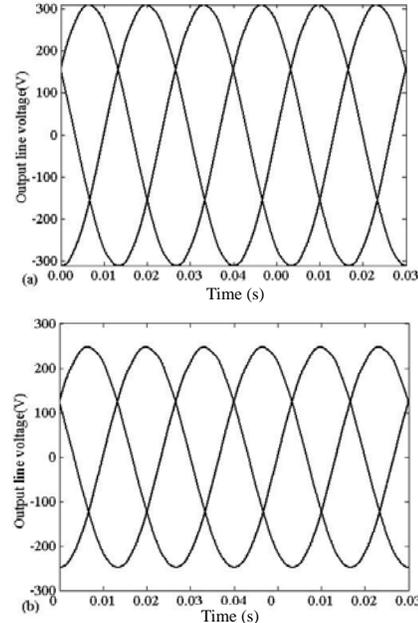
Fig. 6. Output line voltage when  $m \leq 1$ : (a)  $M=1$  and (b)  $M < 1$ .
